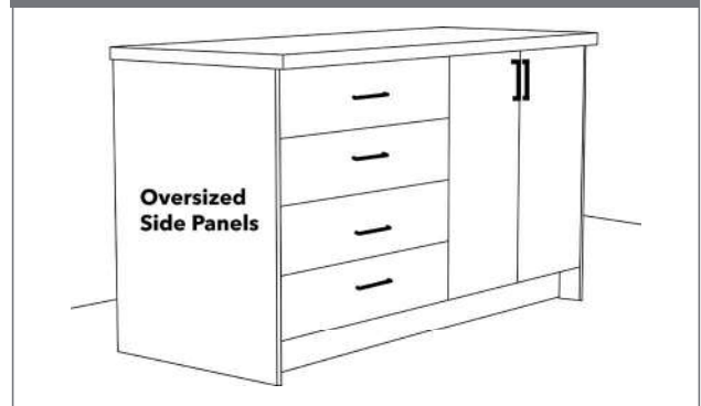
FIG 1.2: FINISHED SIDE PANELS
